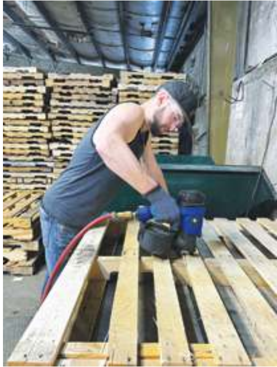
Production Associate Lukas Hood uses a pneumatic nail gun to assemble a pallet.
