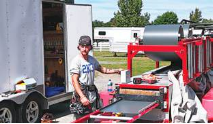
Daniel Tetreault of 2K3 Standing Seam Specialist uses a roll former machine (L), which enables fast and efficient on-site production of standing seam roofing panels. Below, he works on a starter panel.
