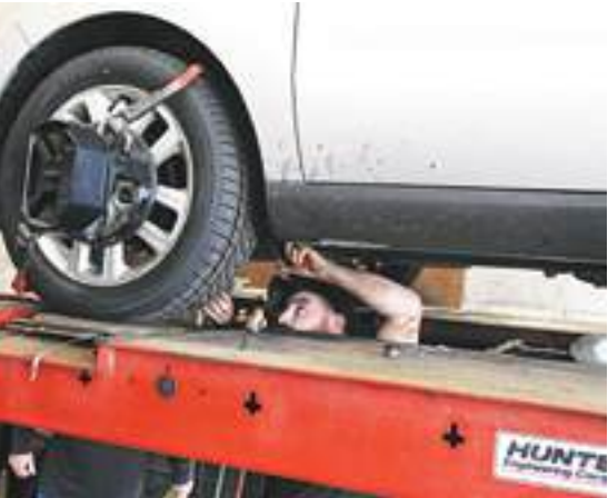
One of two lead mechanics at Dube's Tire Center, Chris Murphy, is pictured executing an alignment.
